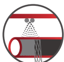
Mesh Wrap & Concrete Coating
